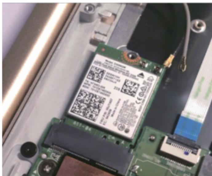
4. Insert the new adapter and install antennas.
