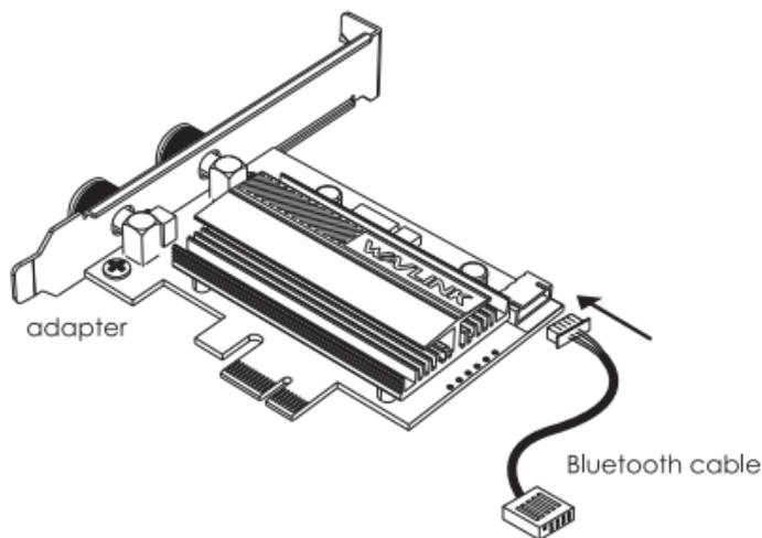
3. Find the corresponding PCI-E slot, then inset the adapter carefully.
